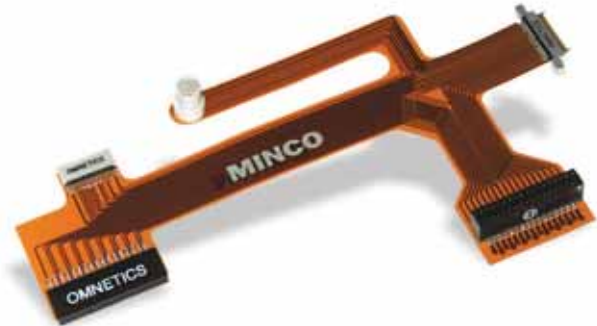
Design hi-rel interconnects with Minco flex-circuits and Omnetics connectors.
